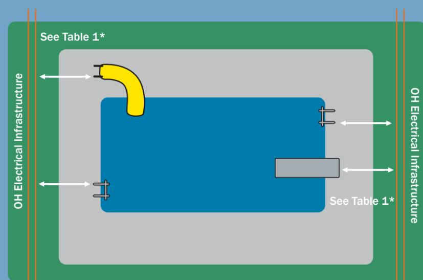
\* From closest point from the electrical equipment to the edge of the pool and pool accessories or unfixed equipment, e.g. diving board, hand rail, slide
